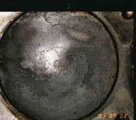
In the same test series, the piston tops shown at the left were from an identical engine burning fuel treated with DurAlt® Fuel Conditioner (FC). Note the lighter deposits which led to an ORI that was lower by 67% than the engine shown at the far left.
